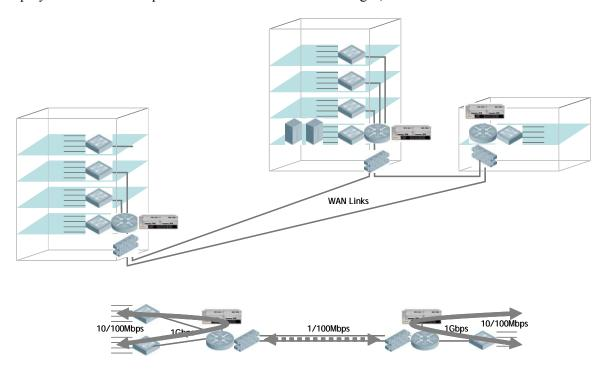
Where locations are large enough to require an on-site Mobility Controller, the model is as suggested above. Each site is provisioned with access points and a local Mobility Controller (or a network of controllers), terminating the control plane. Management is still provided centrally from the mobility management system. Traffic patterns on the data path are unchanged from a wired network.
